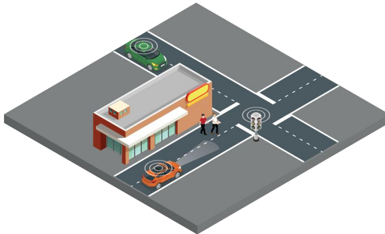
Collision avoidance alert concerning pedestrian sent via V2I and V2V communication.
